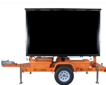
#2427 MESSAGE BOARD SOLAR POWERED 126" X 76" FULL MATRIX
