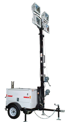
#2110 LIGHT TOWER 4K WATT DIESEL 0.47GPH | 30 GALLON 64 HR. RUN CAP.
