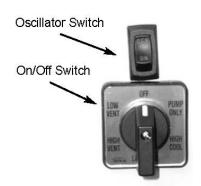
OFF - Power is off to the blower motor and the pump motor.
